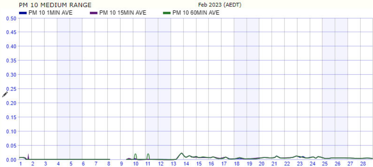
Figure 1. Summary of PM10 from the real time monitoring at location 005 – Solar Industry for the month of February 2023.
