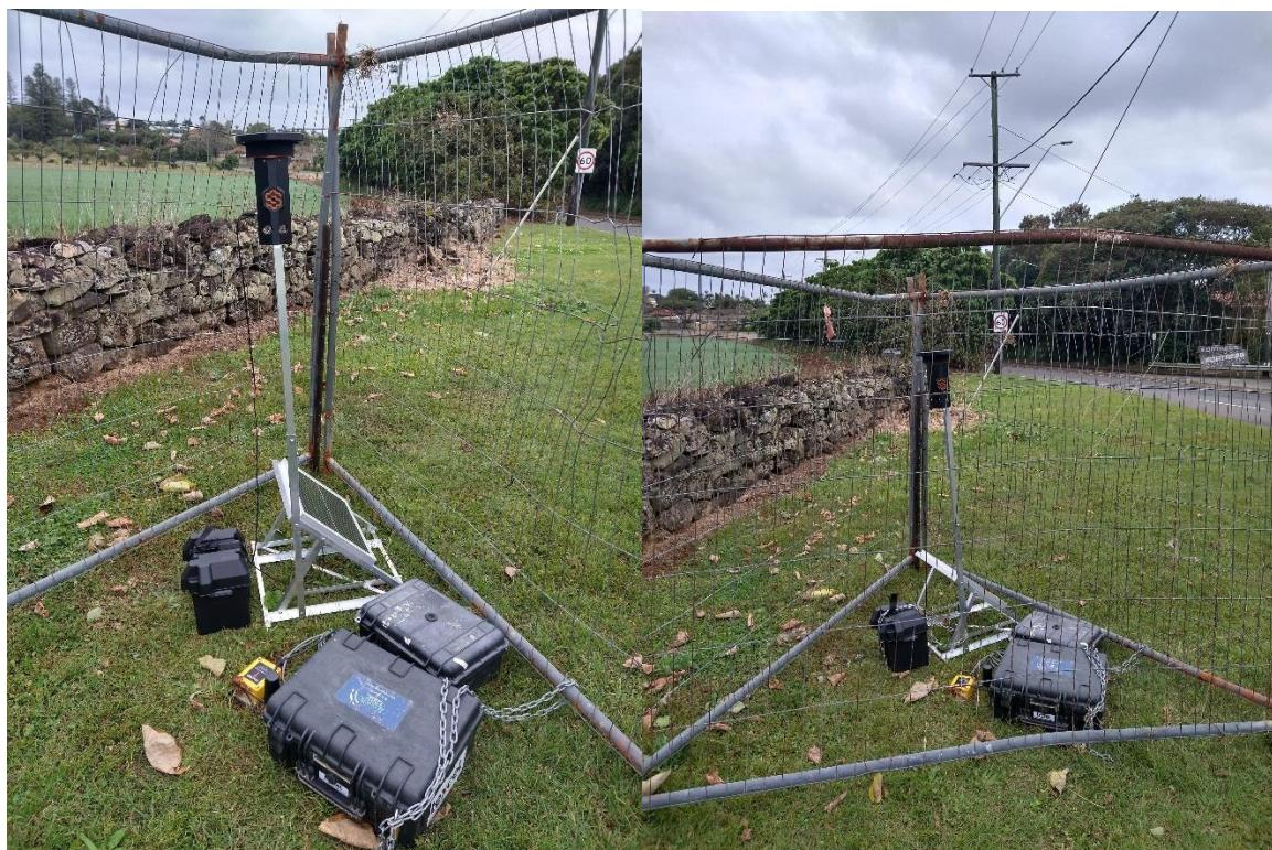
**Figure 3-1 Noise, Dust and Vibration Monitor Installation Locations**
